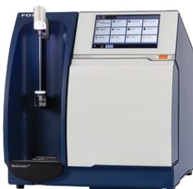
BacSomatic™ is the first-ever integrated bacteria and somatic cell tester. It offers full automation for minimal reagent handling and consistent test results. BacSomatic is easy to use and a fast alternative to manual assay, providing instant, simultaneous results for bacteria count and somatic cell count within 9.5 minutes and 15 samples/hour (1.5 minutes and 40 samples/hour for somatic cell count alone). FDA/NCIMS and EURL/Microval approved.
