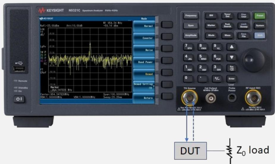
Figure 3. Simple test setup with N9321/22C BSA
