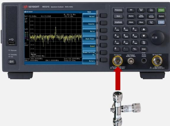
Figure 6. Performing open-short-load calibration on the N9322C BSA
