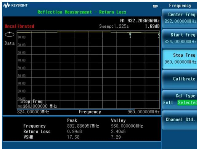
Figure 5. Reflection measurement mode waiting for OSL calibration
