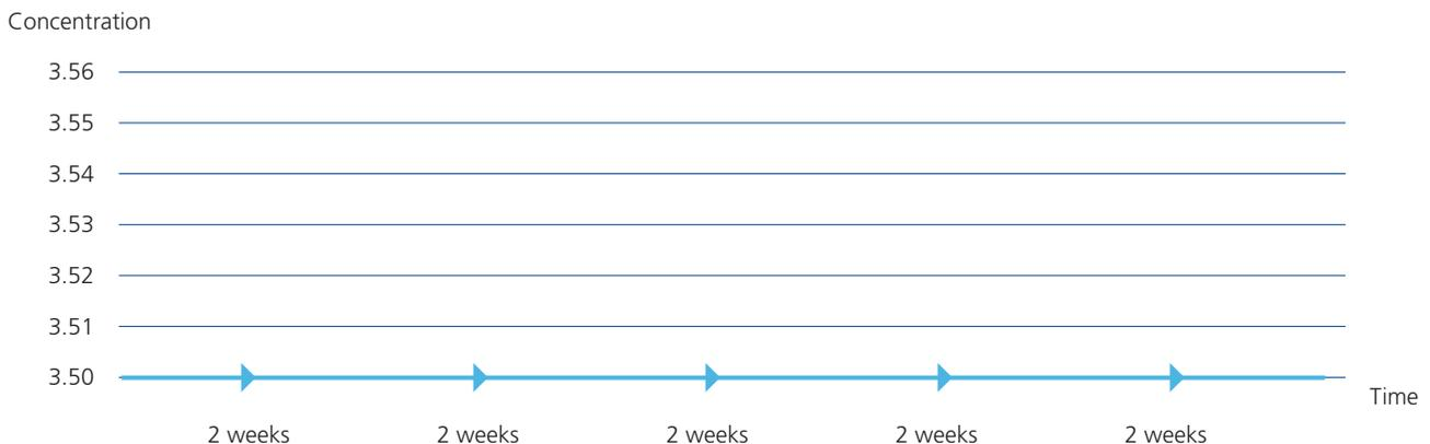
MilkoScan™ FT3 performs an automatic standardisation every two hours that ensures the instrument cannot drift, i.e. results are stable over time.
