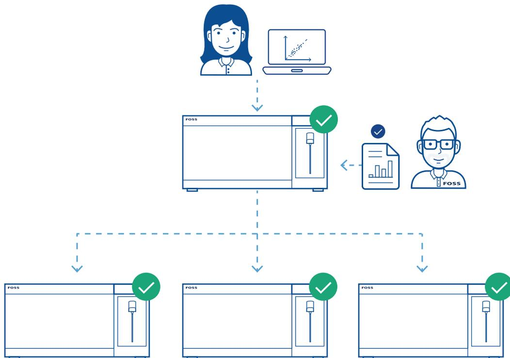
*Excellent transferability ensures that all instruments are the same and that calibrations can be shared in a master/satellite set-up, saving time and money on managing calibrations.*
