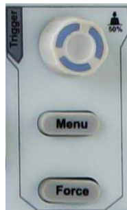
Figure 3-13 Trigger Control Zone
